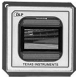
Figure 2.23 Schematic illustration of micromirrors to direct light as desired through electrostatic actuation. Courtesy: Texas Instruments (used with permission).
