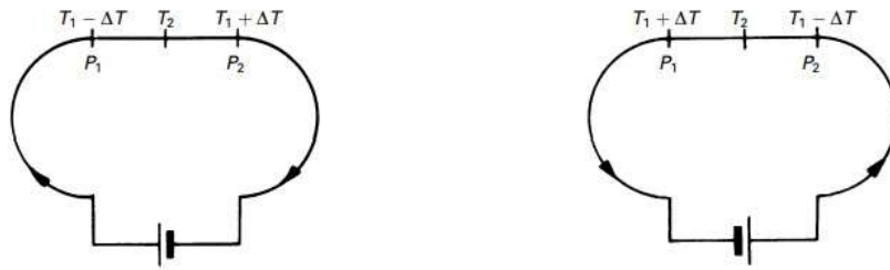
Figure 6.3 Thomson effect: When there is a current along a conductor with non-homogeneous temperature, heat is absorbed or liberated.
