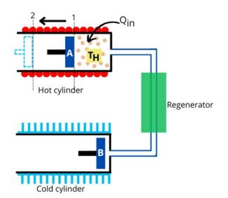
The unit shown in the above figure will help to understand the different processes that occur in the Stirling cycle. It consists of a hot cylinder at temperature  $T_H$ , a cold cylinder at temperature  $T_L$ , and a regenerator.
