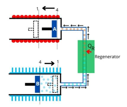
During this process, the air inside the cold cylinder is transferred to the hot cylinder through the regenerator.
