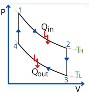
The amount of heat added during the process 1-2 is given by,
