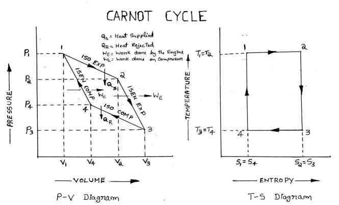
$T_1 = T_{max}$ is the maximum temperature of the cycle $T_3 = T_{min}$ is the minimum temperature of the cycle
